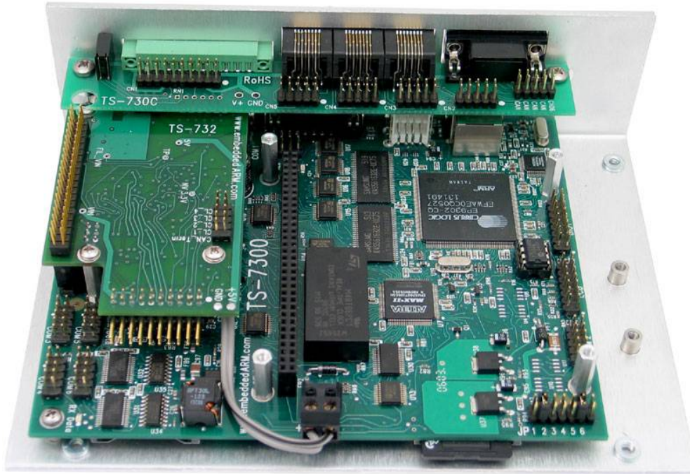
Internal view of TS-ENC730 shown with TS-7300, TS-732 and TS-730C
