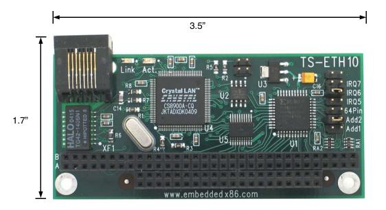
I/O address selection I/O Address <u>Add1</u> <u>Add2</u> Off Off 0x300 Off 0x310 On Off 0x320 On On On 0x330
