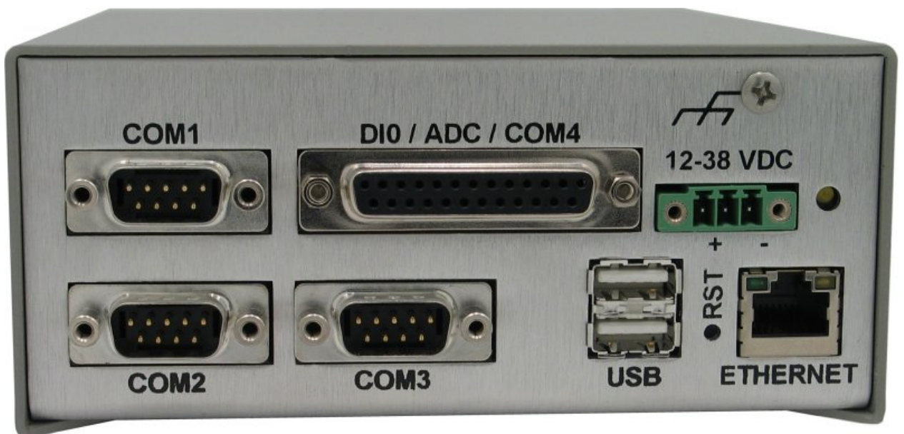
Enclosure TS-ENC550 Rear Panel View
