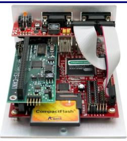
TS-ENC720 shown with optional TS-7200 SBC, TS-CAN1 peripheral board; included cables and TS-782 peripheral board
