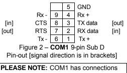
for the RS -232 port and the RS -485 port on the same 9 pin connector, only one of the two functions will be used at a time.
