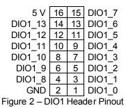
DIO1\_12 and DIO1\_13 are always inputs. In all cases, when a control bit is a "1", it is setting the corresponding DIO lines to be Outputs, while a "0" sets them to be Inputs. All control bits at I/O location Hex 7A are initialized at reset to be "0". When bit 7 of I/O location Hex 7A is a "1", DIO1\_13 is connected to IRQ7 allowing this port to trigger an interrupt.
