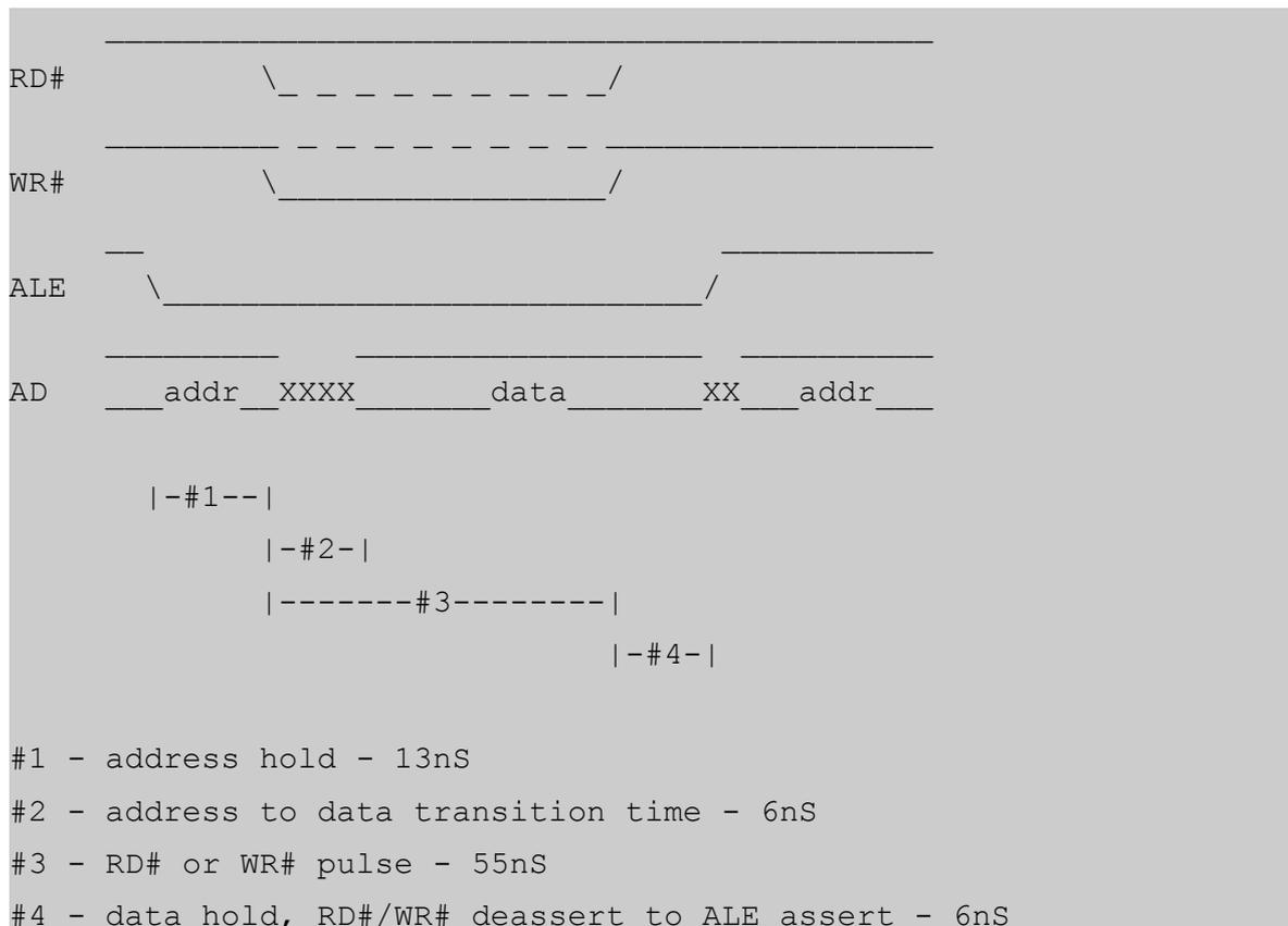
The above timing should be compatible with a standard 74HC373 octal latch chip should you wish to de-multiplex the address/data bus into something more similar to ISA/PC104 externally. If you have questions about whether a particular design will work or not, please feel free to contact Technologic Systems with your schematic for review.
