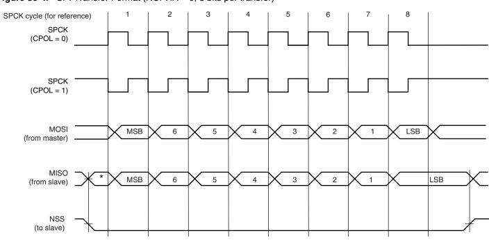
**Figure 30-4.** SPI Transfer Format (NCPHA = 0, 8 bits per transfer)
