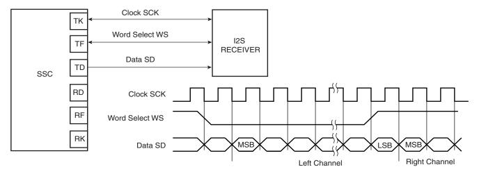
Figure 33-18. Codec Application Block Diagram
