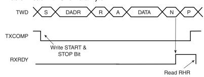
Figure 31-10. Master Read with Multiple Data Bytes
