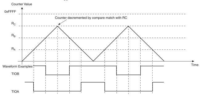
Figure 34-14. WAVSEL = 11 With Trigger
