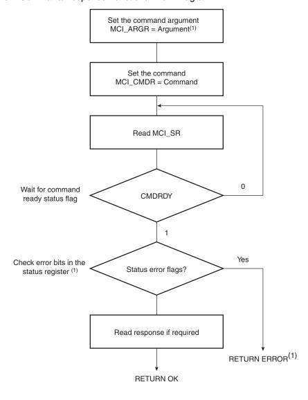
Figure 35-9. Command/Response Functional Flow Diagram
