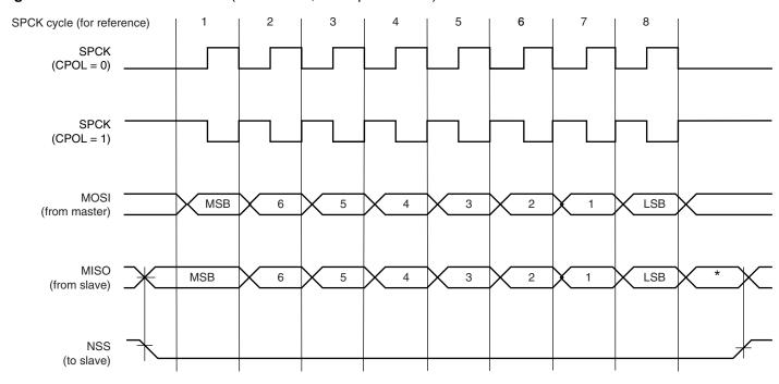
Figure 30-3. SPI Transfer Format (NCPHA = 1, 8 bits per transfer)
