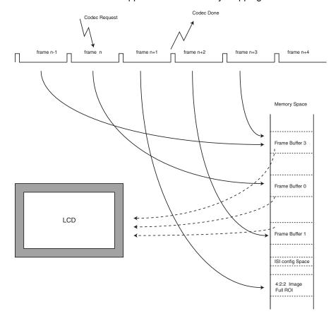
Figure 39-6. Three Frame Buffers Application and Memory Mapping
