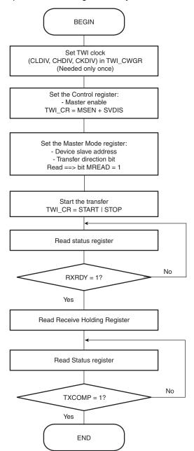
Figure 31-18. TWI Read Operation with Single Data Byte and Internal Address
