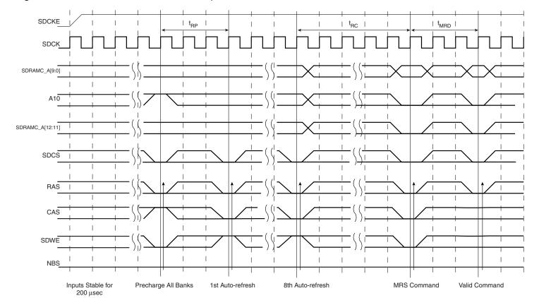
Figure 22-1. SDRAM Device Initialization Sequence
