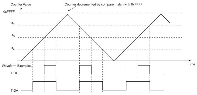
Figure 34-12. WAVSEL = 01 With Trigger
