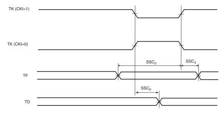
Figure 41-15. SSC Transmitter, TK and TF in Input
