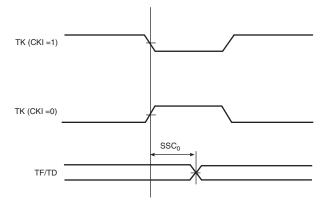
Figure 41-13. SSC Transmitter, TK in Input and TF in Output
