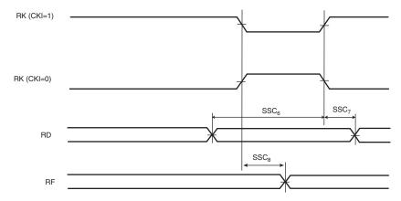
Figure 41-18. SSC Receiver, RK and RF in Output
