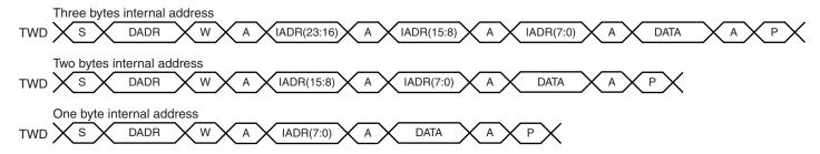
Figure 31-12. Master Read with One, Two or Three Bytes Internal Address and One Data Byte
