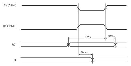
Figure 41-19. SSC Receiver, RK in Output and RF in Input
