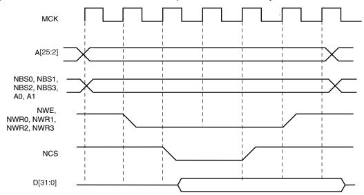
Figure 21-15. WRITE\_MODE = 0. The write operation is controlled by NCS
