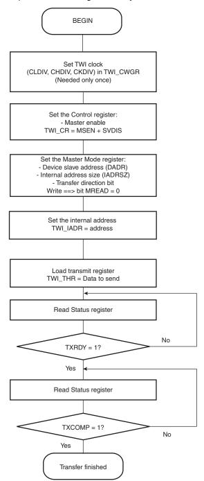
Figure 31-16. TWI Write Operation with Multiple Data Bytes with or without Internal Address
