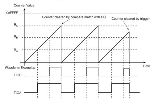
Figure 34-10. WAVSEL = 10 With Trigger
