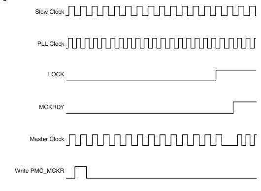
Figure 26-4. Switch Master Clock from Main Clock to Slow Clock
