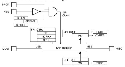
Figure 30-9. Slave Mode Functional Block Diagram
