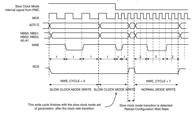
Figure 21-34. Recommended Procedure to Switch from Slow Clock Mode to Normal Mode or from Normal Mode to Slow Clock Mode
