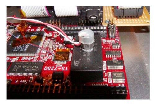
With the testing equipment all in place, the four TS-7250 boards were subjected to stress conditions using repeatable testing techniques such as thermal step stress, rapid thermal transitions, vibration step stress and combined temperature and vibration environments. These testing cycles create conditions that quickly reveal weaknesses in the product design and failure modes.
