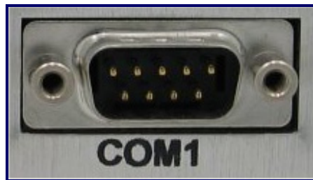
Enclosure TS-540 COM1 Port
