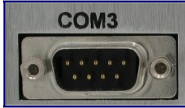
Enclosure TS-540 COM3 Port
